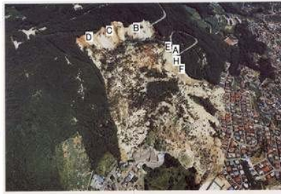
Fig.1 Jizukiyama landslide in Japan (26 Sep. 1985) (Nagano pref.,1985) (A to H : location of extensometer)
