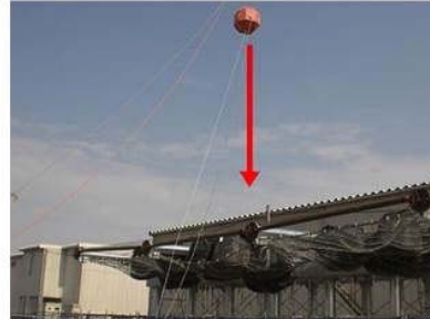
Load test for Impact force
