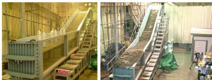
Performance test using landslide flume with artificial rainfall at FFPRI
