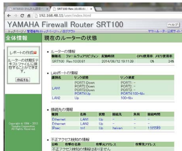
Figure 4 (Screen Shot)The management screen that you see through the VPN from the Vietnam side of the Japanese side (YAMAHA SRT-100(Japanese setting)).
