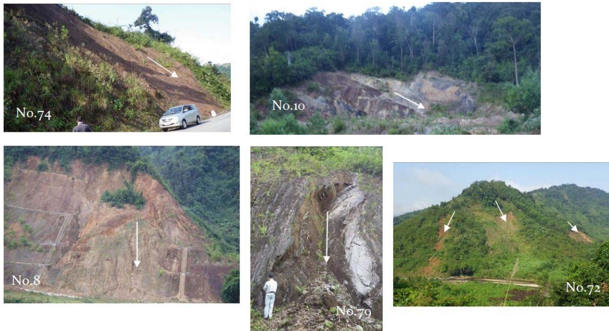
Figure 5 Moving types of landslides along HCMR ( No74: Translational shallow debris slide, No.10: Translational rock slide, No8: Rotational slide, No.7: Translational wedge type slide, No.72: Gully type slide and flow)
