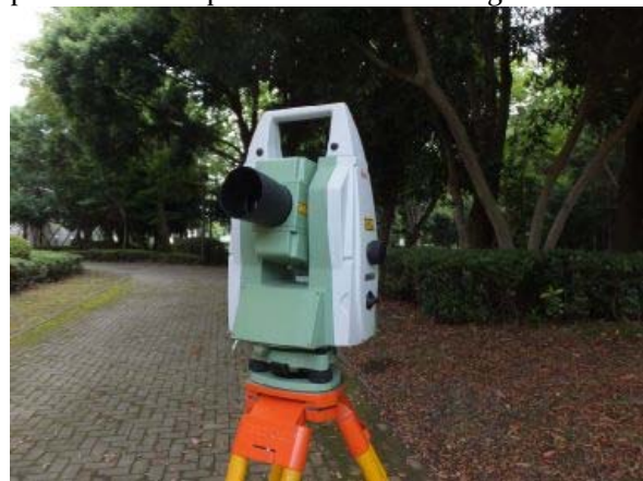
Photo 2 Robotic total station
