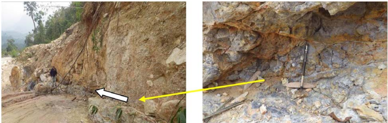
Figure 22 Ancient translational rock slide and slide surface of coal bed (right) -No.357-
