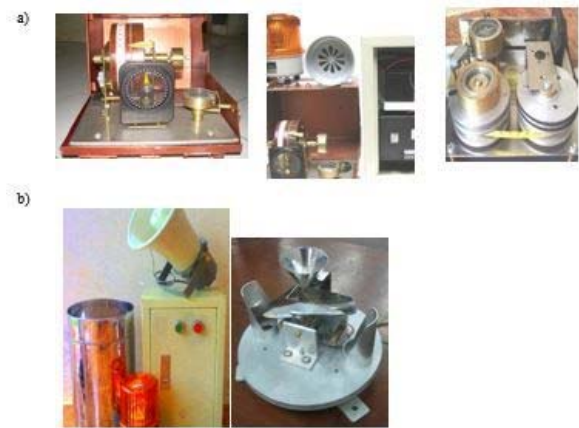
Figure 3a above, the manual extensometer (generation 1 on the left and generation 2 on the right), connected with alarm system in the middle, stem in the middle, and 3b below, the rain gauge with the alarm system (Fathani et al, 2008; Fathani and Karnawati, 2009).
