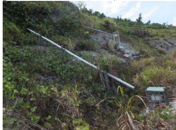
Photo 4 Extensometer of short span type in Hai van
