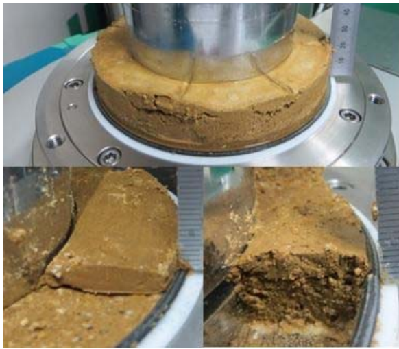
Figure 13 Sliding surface liquefaction and grain crushing in the shear zone in ring shear test
