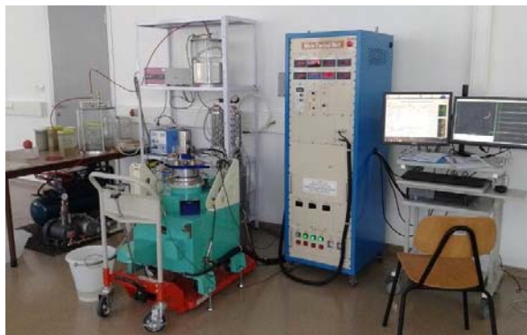
Figure 8 New developed portable ring-shear apparatus designed for testing under static and dynamic conditions for deep-seated large landslides in Croatia.
