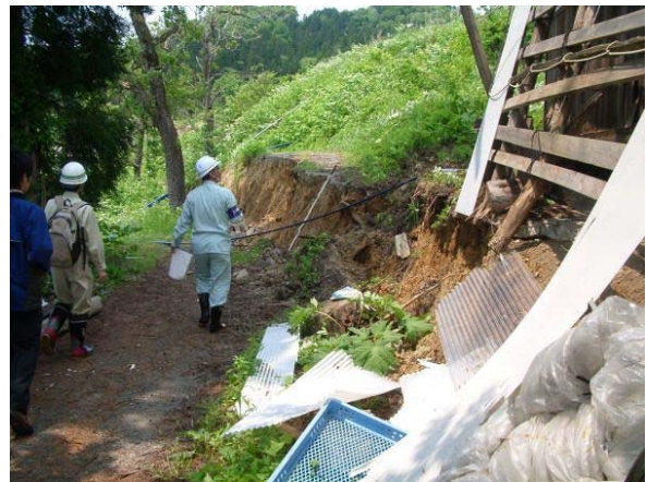
Figure 4 Main scarp at the top of slope (Taken by Landslide Research Team, 2009)
