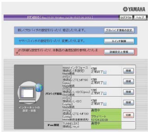
Figure 5 (Screen Shot)Japanese side staff indicates a management screen that referenced Vietnamese router (YAMAHA RTX-810(Japanese setting)) through the VPN.
