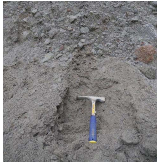
Fig 3 Photo of the sand layer behind hammer from which sample (S 1 ) was taken. It is exposed in the bank of a torrent gully in the source area of the Unzen-Mayuyama landslide
