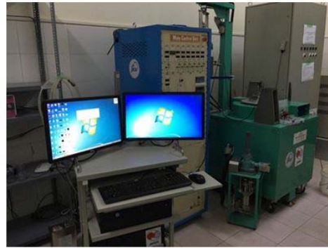
The New High Stress Undrained Ring Shear Apparatus (ICL-2) (International Consortium on Landslide)
