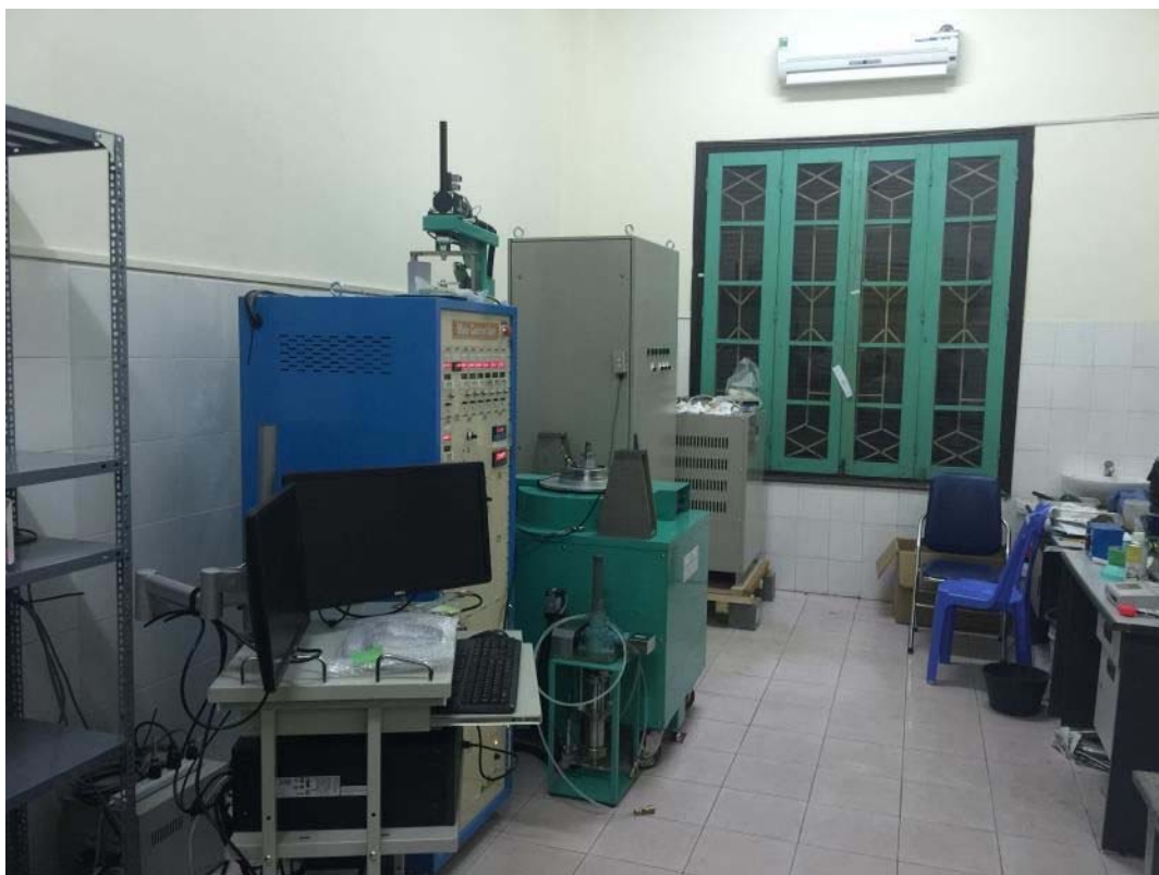
Fig 7. Pictures of a high-stress undrained dynamic loading ring shear apparatus (ICL-2) in Lab. ITST, Vietnam
