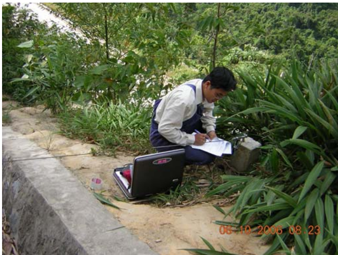
Figure 14 Checking the data of extensometer
