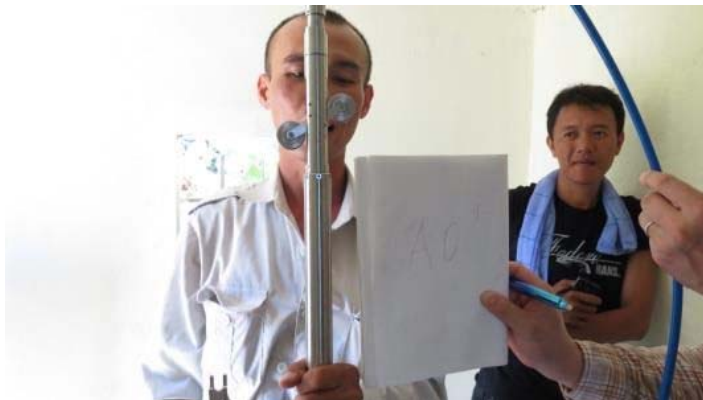
Figure 17: Insert probe inclinometer in A_0 - A_{180} direction
