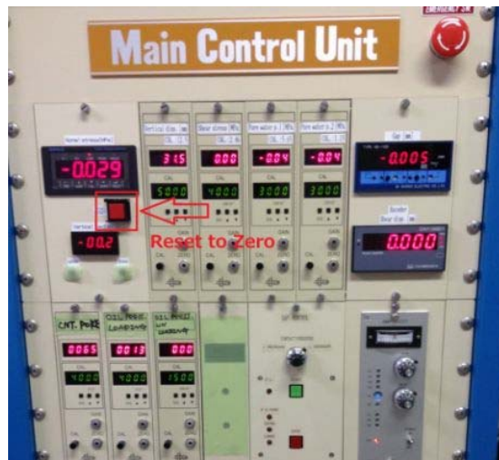
Fig. 6 Reset Gap value to zero
