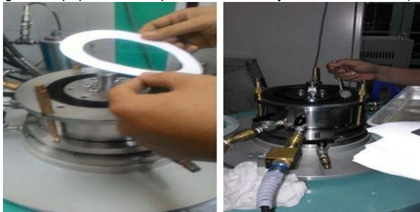
Fig. 12 Putting a filter paper and building the sample
