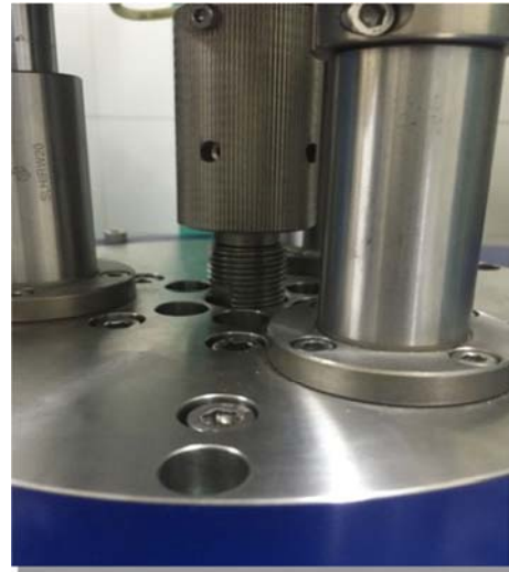
Fig. 22 Disconnection of VLC and central axis
