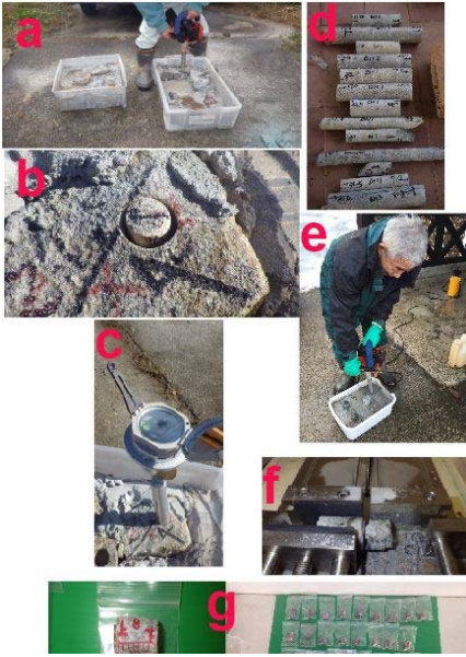
Fig. 9 Sampling and shaping of remanent magnetism measurement specimens: a, b, c, specimen gouging from exposed rock fragments; d, e, drilling core samples and specimen gouging; and f, g: shaping and completed specimens.
