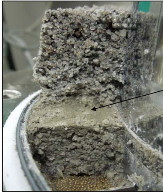
Fig. 24 Shear zone is presented by a black arrow
