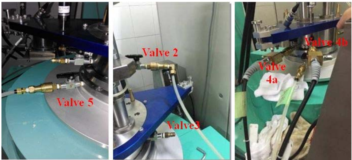
Fig. 10 Prodecure of CO 2 and H 2 O Saturation
