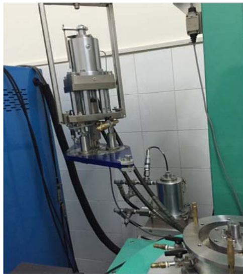
Fig. 23 Reinstalling Loading Plate (the plate in dark blue color)
