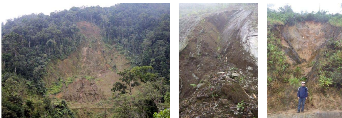
Fig. 5.2 (a)Debris Shallow landslide and (b), (c)Translational wedge type slides in HCMR -Hue section-Vietnam
