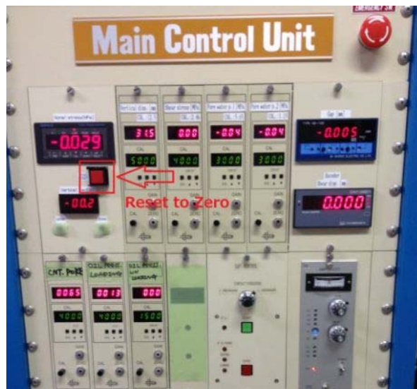
Fig. 6 Reset Gap value to zero
