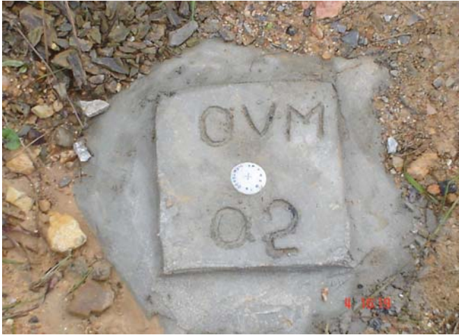
Figure 12 Concrete post for landslide monitoring
