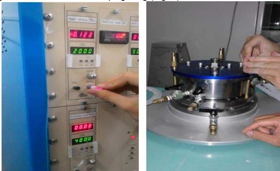
Fig. 8 Increasing Contact pressure and removing the Helping Ring
