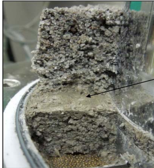
Fig. 24 Shear zone is presented by a black arrow
