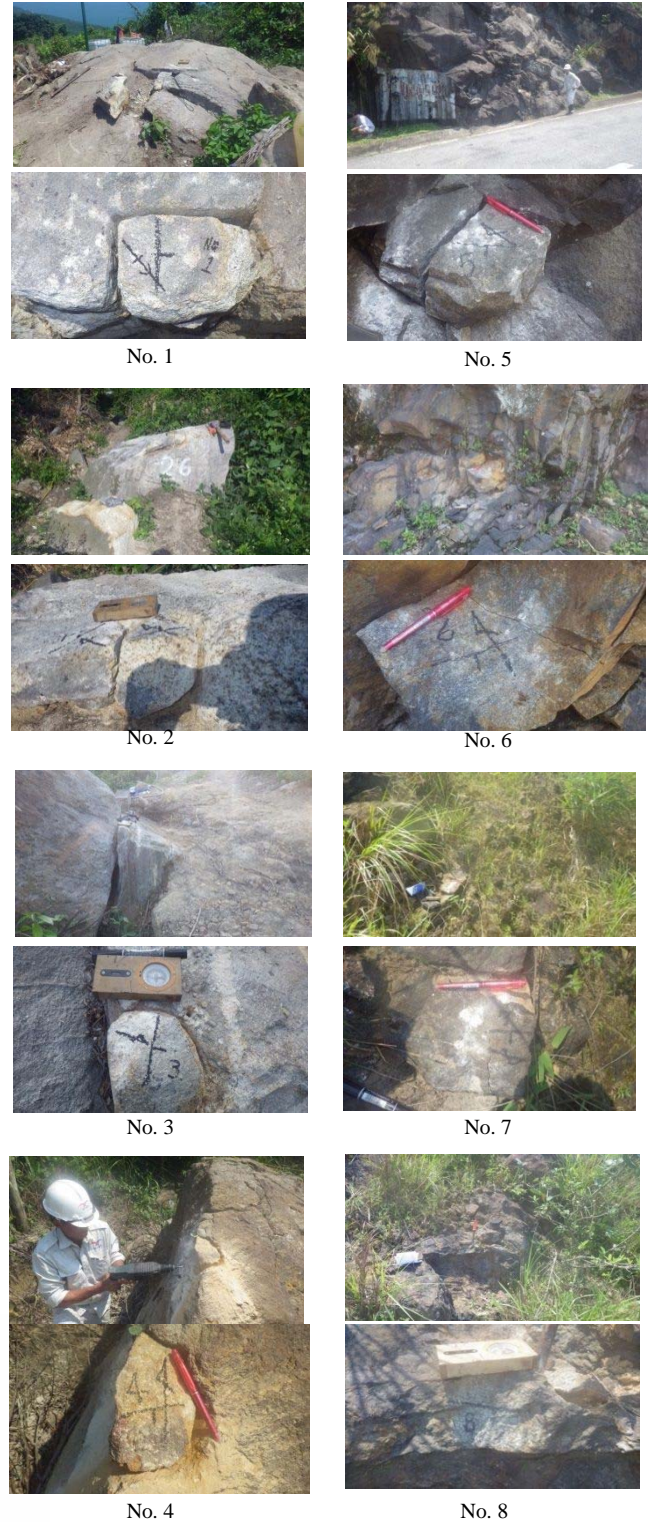
Fig. 8 Sampling of remanent magnetism measurement specimens from exposures
