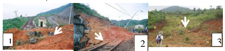
Fig. 4 Recent landslides taking place within the Hai Van landslide: 1–2, Landslide at heavy rain in November, 2007 (Units A, C of Fig. 3). ;3, Landslide at forest road construction site, year unknown (Unit E of Fig. 3).
