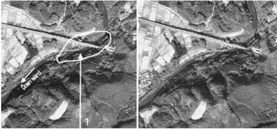
Figure 20 Landslide body and adjacent environment. Landslide body at lower face to the other near. Increase toward the active condition. Weight value: 8.6. Landslide body face to the undercutting slope of river stream has very high potential of landslide (Miyagi et al., 2004).
