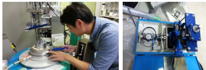
Figure 2. testing RSA with Hai Van sand and potable direct shear test.
