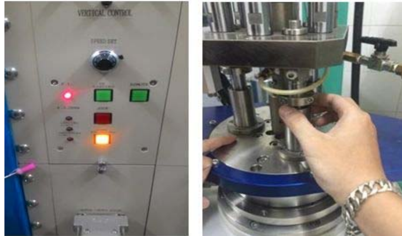
Fig. 15 Install VLC and unlocking the fixers
