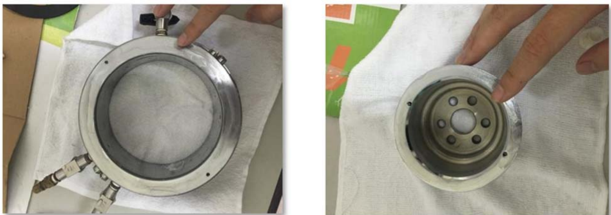
Fig. 3 The inner and outer rings are covered in grease
