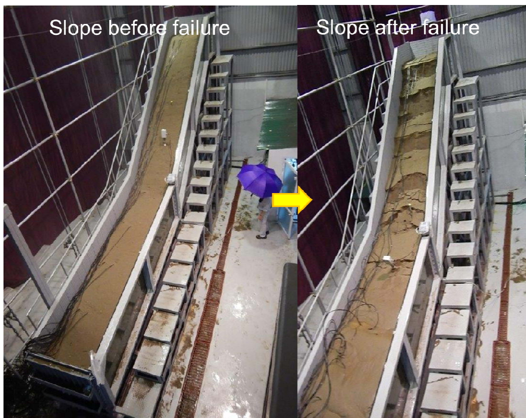
Fig. 4: Slope before failure (left side) and after failure (right side) on flume experiment in ITST (Hirotaoka Ochiai et al., 2016)
