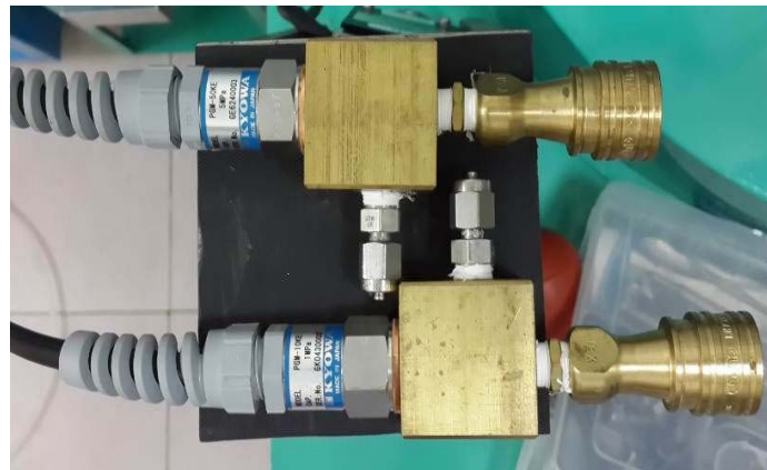
Fig. 11 A photograph of pore water pressure transducers PPT-1, PPT-2
