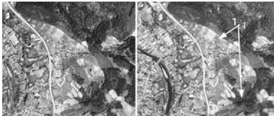
Figure 14 Major boundary of landslide. This is the case of suspended landslide. There is talus topography (1) developed between the main scarp and the body. The weight value is 1.8 (Miyagi et al., 2004).
