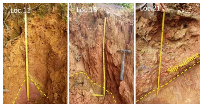
Fig. 4 Identify slip surface at the landslide site along Ho Chi Minh Road (Aug, 2013)
