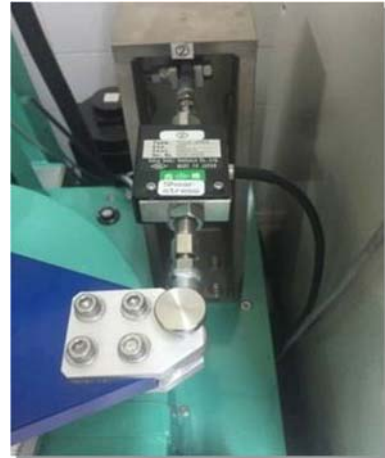
Fig. 14 Installing Shear Load Cells
