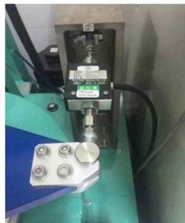
Fig. 14 Installing Shear Load Cells
