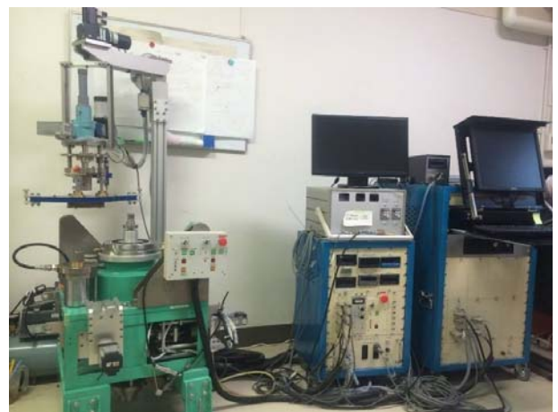
Fig 1. General view of the portable ring shear apparatus, ICL-1
