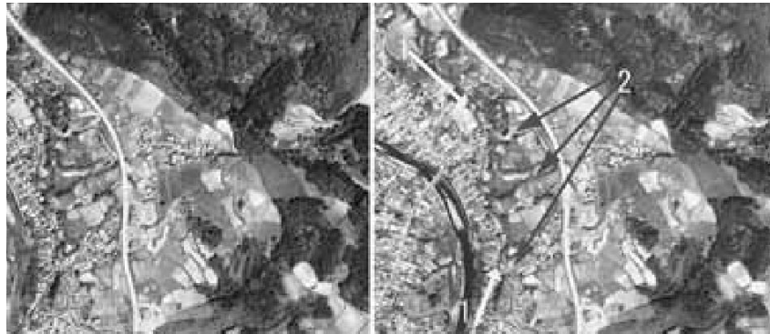
Figure 13 Gullies development. Weight value: 3.6. The normal erosion processes will appear at the suspended stage. Gully erosion is one of the clear and easy to interpretational features. 1; Lateral erosion by stream cut the toe part of the body. 2; Gullies start the dissection to the toe part of body (Miyagi et al., 2004).
