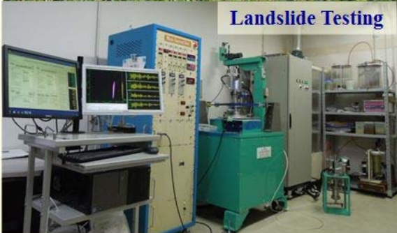
A dynamic loading undrained ring shear apparatus to measure landslide dynamics parameters
