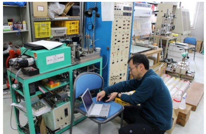
Fig. 8 Residual strength characteristics of weathered rocks were conducted in the laboratory in Fukushima, Japan (Dung et al., 2016 submitting).
