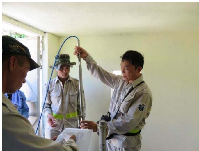
Figure 18: Rotary 180^\circ to teke the Wheel on the probe intro Channel A_{180}
